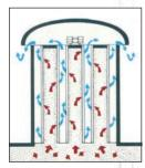
Untreated gas flows into the filter hoses that are open at the bottom and closed at the top. Clean gas escapes between filter housing and weather-hood.
