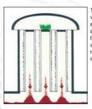
The imbalanced vibrator is activated either manually or automatically and the hose surfaces are cleaned. The material flows back into the silo.
