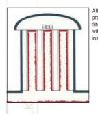
After the filling process the hose filter unit is coated with dust on the inside.
