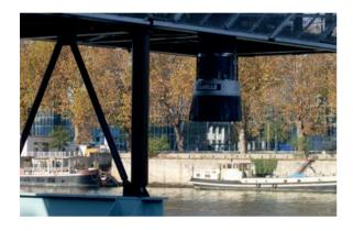
The Stanelle JET loaders TYPE RONDO 350 / 400 / 500 with an extended hub are designed for loading ships and slagheaps. The required volume of exhaust air of approx. 2,000 - 3,000m³/h can be extracted via the suction nozzles by using an appropriate dedusting unit.
