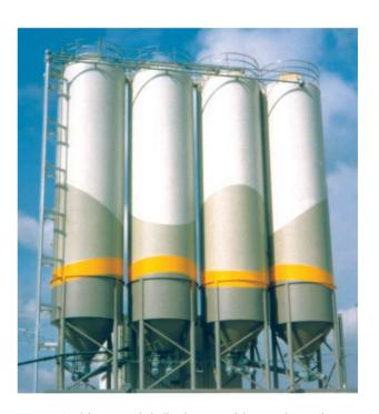
supported by special discharge aids, such as the Stanelle LUALO air injection fluidisation system or the ASK discharge vibrating cone.
